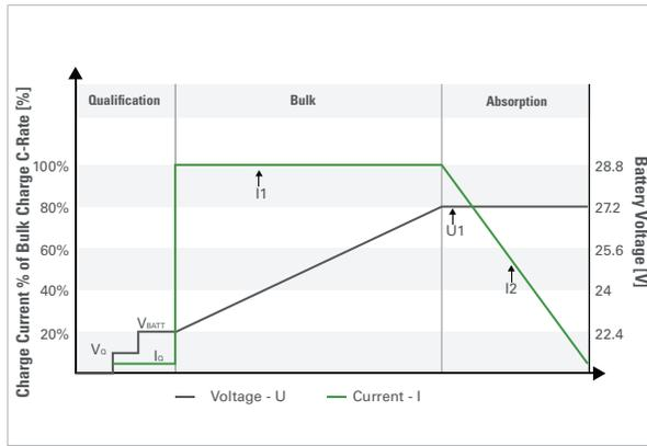
**VOLTAGE REGULATED IU CHARGING CURVE PARAMETERS**
